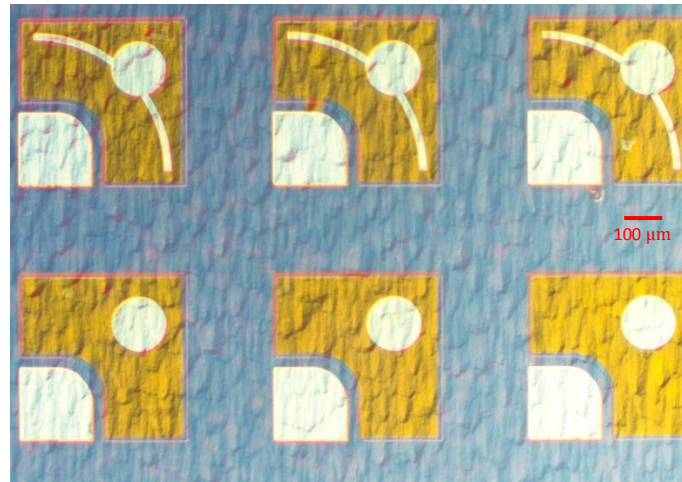
Successful formation of n-contacts after liftoff
